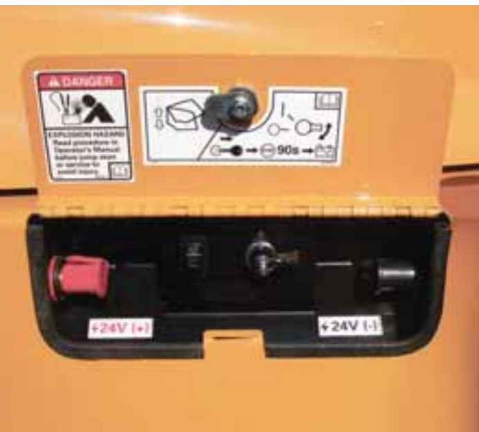
Hood opening and battery on/off switches. In case of flat battery, hood opening can be done externally with remote jump start
